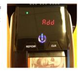
b. "Bill Exit Direction" – A small green arrow points to either the front or the back of the unit. This arrow indicates where bills will be "exited" from the CT550. Bills may either be exited from the front or the rear of the unit, depending upon user preference. The direction can be changed by simply pressing and holding the ""REP/DIR" button until the unit beeps and the direction of the green arrow changes.
