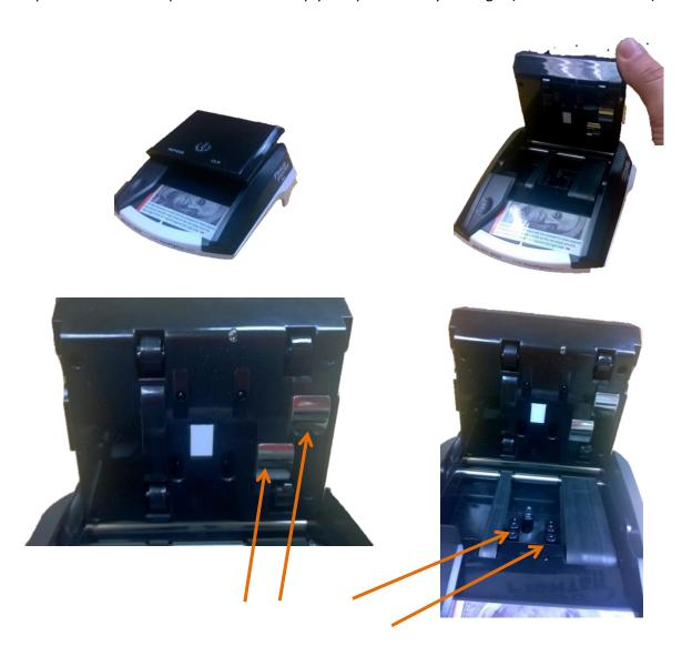
For best results use rubbing alcohol or a light cleaner that will not leave a residue (such as a glass cleaner) and wipe the wheels, optical and metal magnetic sensors (note arrows) on the top and bottom. Clear any dust from inside and also wipe the belts if needed. It is also effective to use compressed-air type electronic cleaners to blow dust off these surfaces. Close the lid and make sure the top snaps all the way down. If any questions please call 800.883.8822
