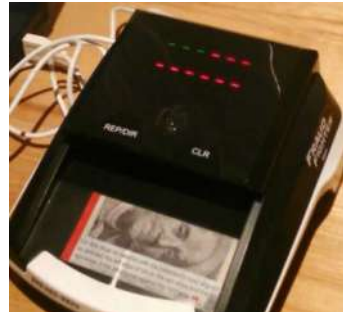
Twelve dashes should appear on the display window in “download mode”.
