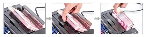
**Note!** Some people find it easier to select "manual" which allows the user to properly align the banknotes in the feeder hopper, and THEN press "start" to initiate the counting.
