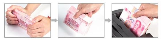
**Second Method:** Place stacked notes leaning forward into the hopper area, "tilt" the notes back so that the slide gently into the hopper feeding area.
