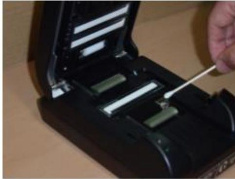
*Figure 26 - Cleaning the magnetic stripe reader*
