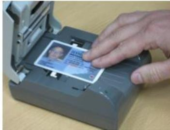
*Figure 32 - Removing a jammed document from scanner*
