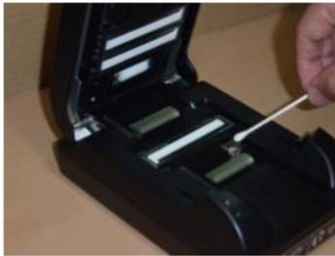
*Figure 28 - Cleaning the magnetic stripe reader*
