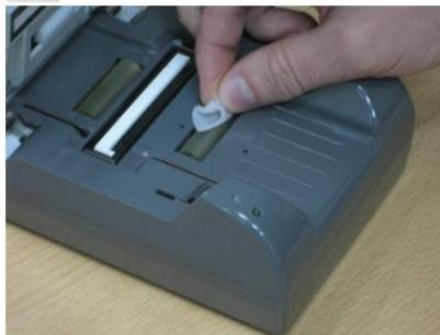
Figure 26 - Cleaning the feed rollers
