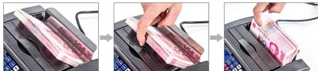
**Note!** Some people find it easier to select “manual” which allows the user to properly align the banknotes in the feeder hopper, and THEN press “start” to initiate the counting.
