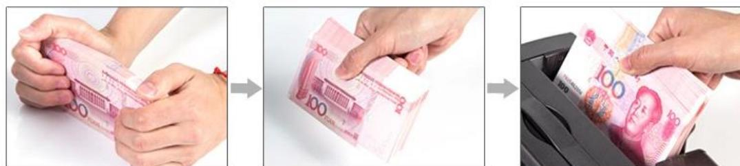
**Second Method:** Place stacked notes leaning forward into the hopper area, “tilt” the notes back so that the slide gently into the hopper feeding area.
